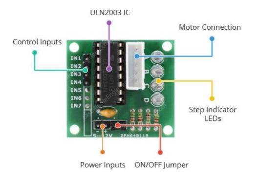
The board has a connector that mates the motor wires perfectly which makes it very easy to connect the motor to the board. There are also connections for four control inputs as well as power supply connections.
