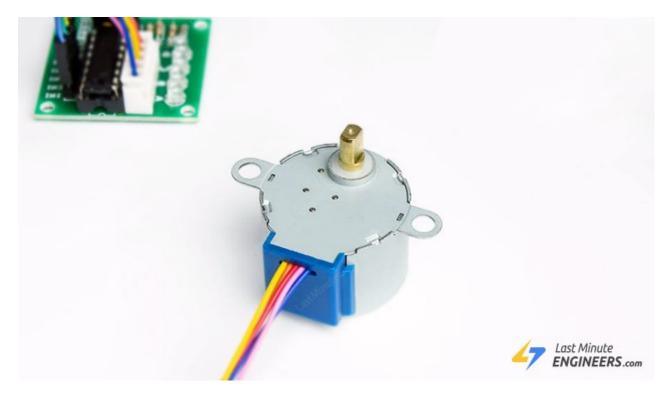
Stepper motors are great motors for position control. They are a special type of brushless motors that divides a full rotation into a number of equal "steps". They are usually found in desktop printers, 3D printers, CNC milling machines, and anything else that requires precise positioning control.
