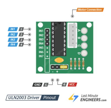
IN1 – IN4 pins are used to drive the motor. Connect them to a digital output pins on the Arduino.
